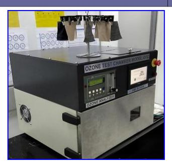
Colorfastness Testing System as per AATCC TM-109 (Optional: as per AATCC TM-129/ISO 105-G03)
